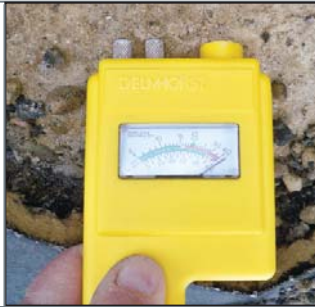
Photo 4. External Probes Determines the depth of moisture
